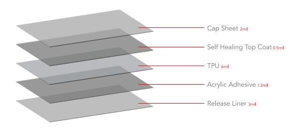
Nominal Thickness Without Liner 195 +/- 10 µm
