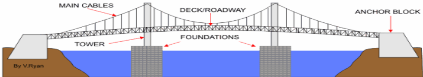
BASIC DIAGRAM - THE AKASHI-KAIKYO SUSPENSION BRIDGE
