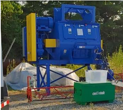
Photo: ceEntek's Model 30 UHPC mixer & vibrating screed set up
