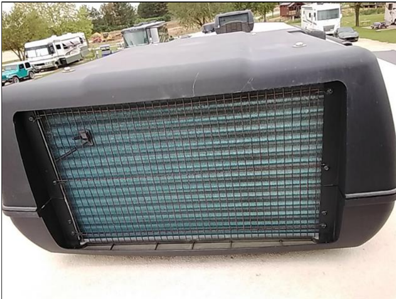
Rear AC Coils
