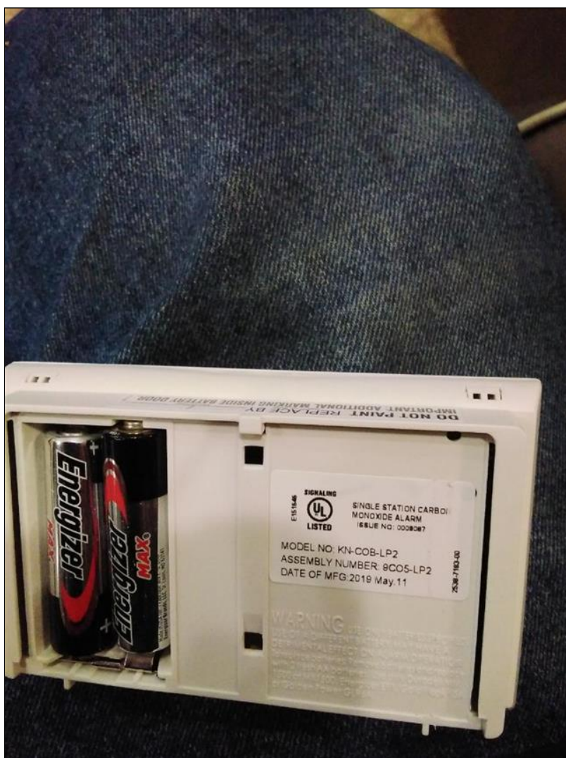
rear plate on carbon monoxide detector
