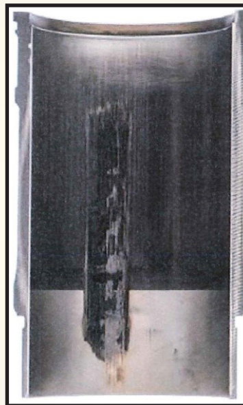
Severely scuffed liner after 47 hours
