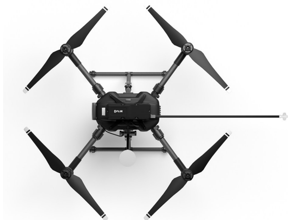
A DRONE SYSTEM WITH A 6 GAS DETECTOR AND PROBE AS ITS PAYLOAD
