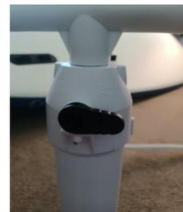
4. Pump the board until you find it hard to pump, then move the lever into the single action position (this will make it easier to pump). Carry-on pumping until you reach 18psi on the gauge. This should take around 15-20 minutes with two people pumping with both pumps supplied.
