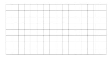
Product No.LengthWidthHole SpacingGaugeMaterial20218'4'6" x 6"10Electro Galvanized
