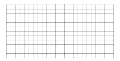
Product No.LengthWidthHole SpacingGaugeMaterial20368'4'4" x 4"8Class 1 Galvanized
