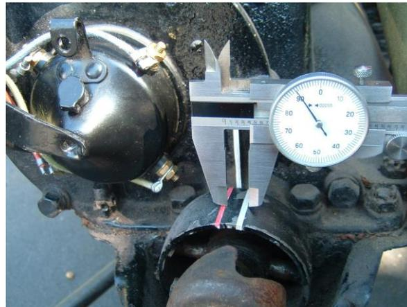
**Figure 6.** Measuring the crank travel between cylinder 1 TDC and cylinder 1 firing position.
