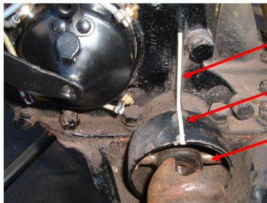
Use masking tape to mark reference line on timing cover
