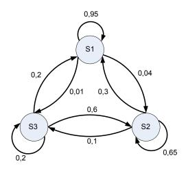
Figure B.9 – Example of system Markov diagram
