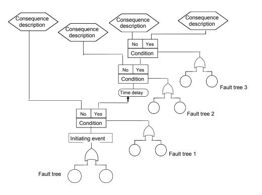
Figure B.4 – Example of cause-consequence analysis
