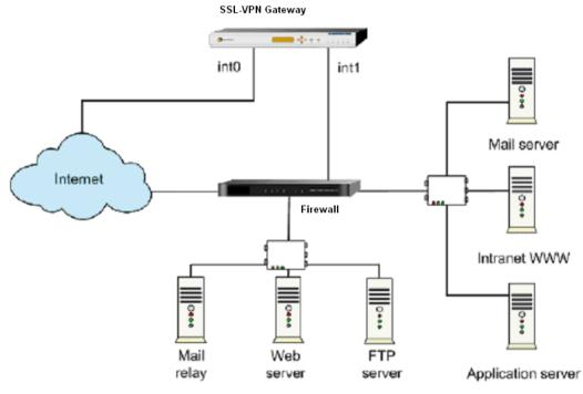
A potential problem of this configuration is that the VPN Gateway is left unprotected by the perimeter security gateway. For example, the VPN Gateway could be susceptible to protocol anomaly attacks or network attacks.
