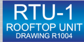
Nameplate Size: 2 x 4 in Row one - 3/4 inch text size Row two - 3/8 inch text size Row three - 1/4 inch text size
