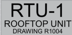
Nameplate Size: 2 x 4 in Row one - 3/4 in text size Row two - 3/8 in text size Row three - 1/4 in text size
