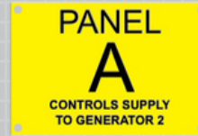
Nameplate Size: 2 x 3 in Row one - 3/8 inch text size Row two - 3/4 inch text size Row three & four - 3/16 inch text size
