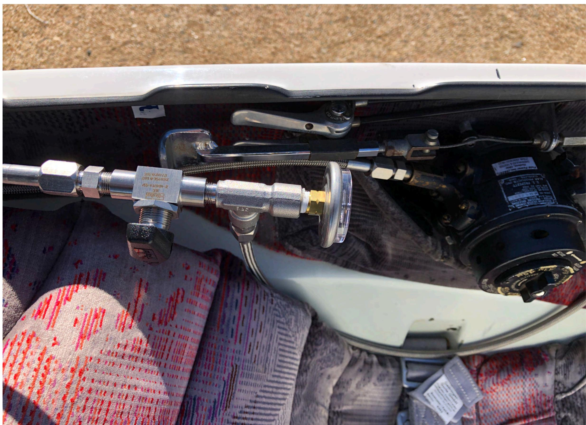
A-14, high pressure hose, valve, and gauge installed in glider.
