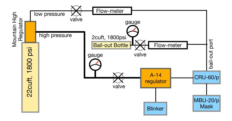
Oxygen circuit: A-14, with fixed-flow and bail-out bottle for backup.
