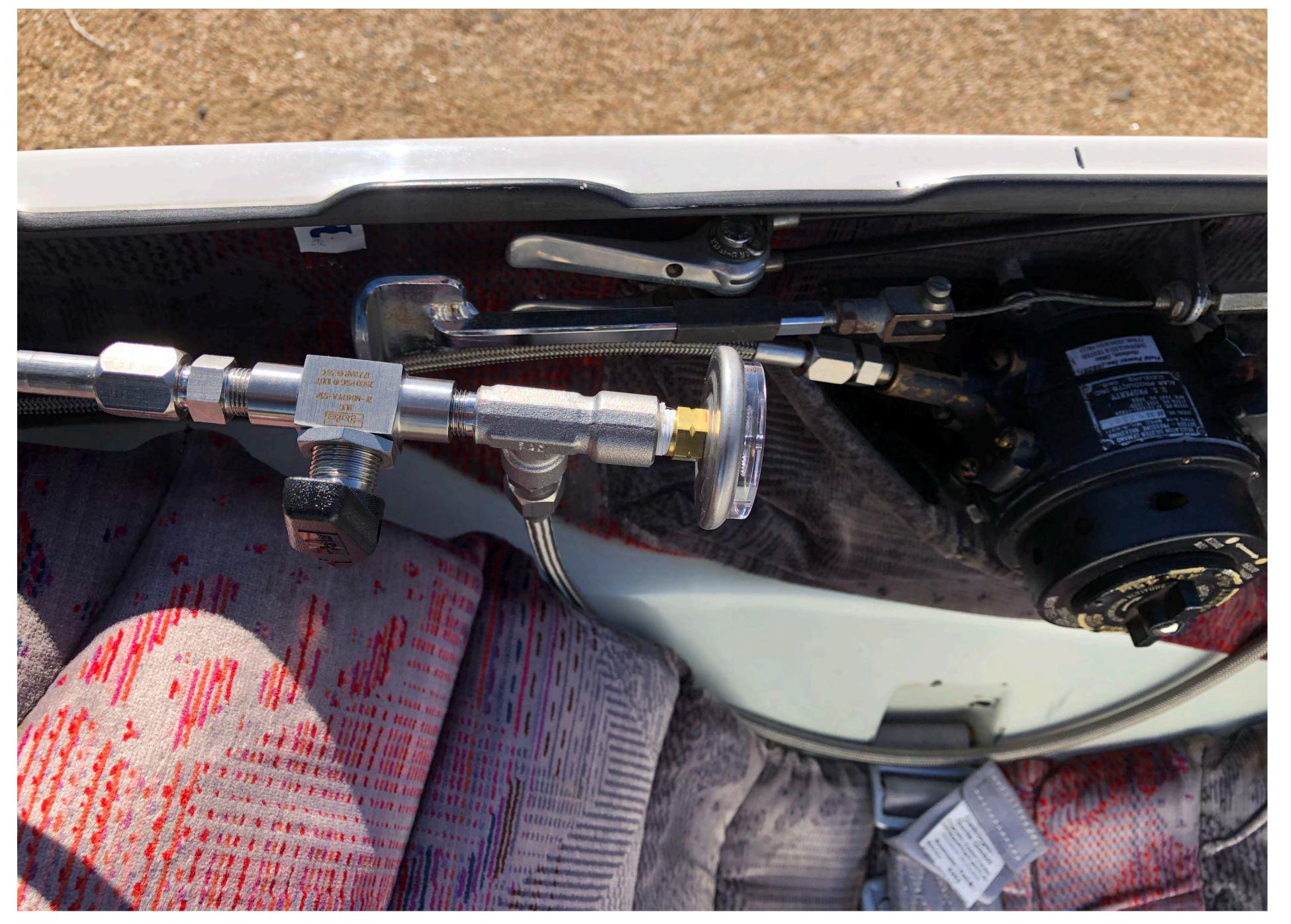
A-14, high pressure hose, valve, and gauge installed in glider.
