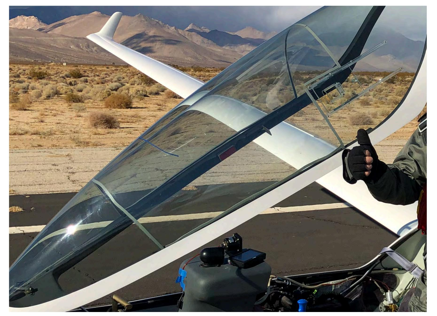
Frost Shield: 1/16" thick polycarbonate, sealed against canopy with weather stripping.
