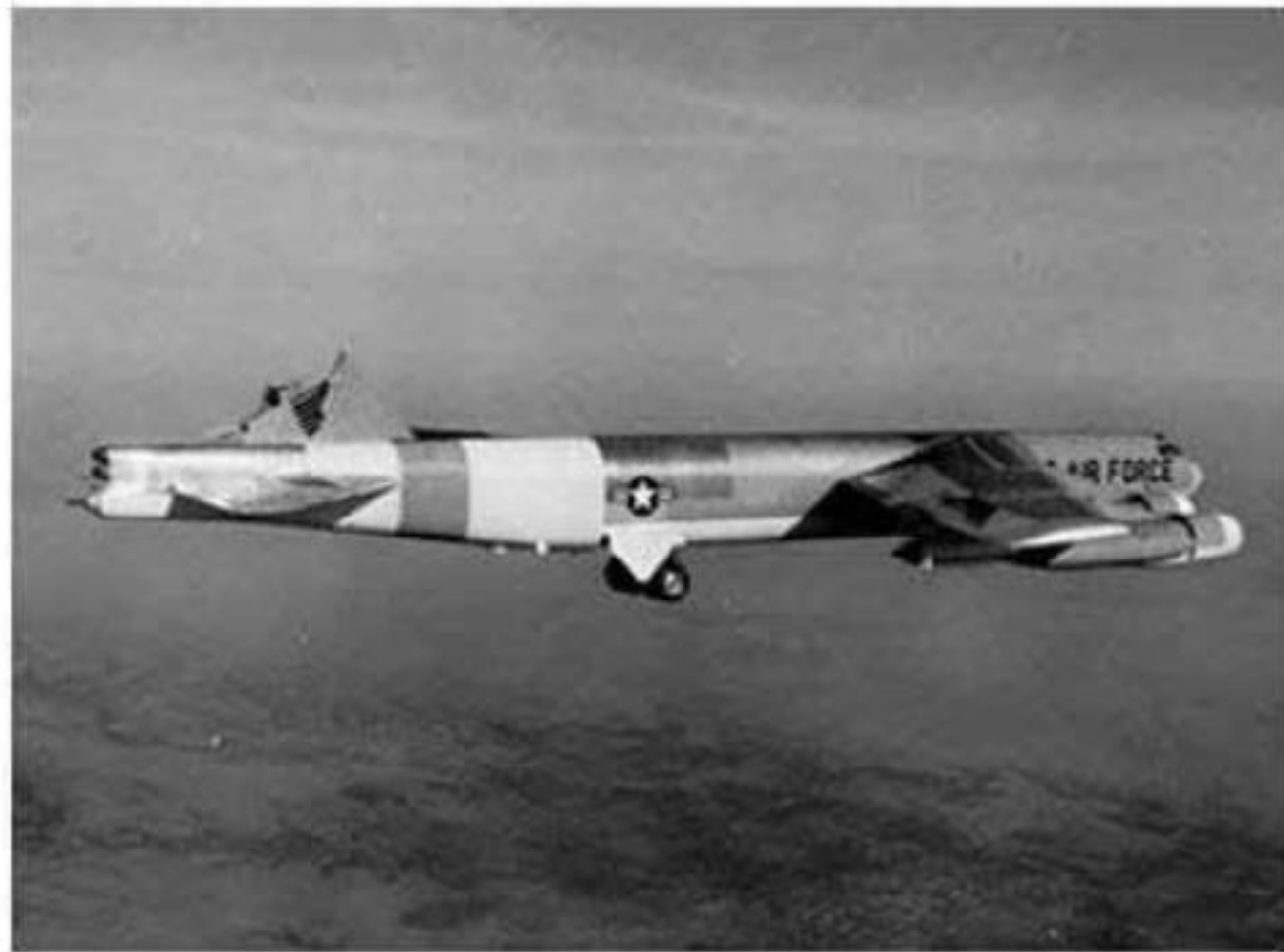
Figure 1: USAF B-52H Stratofortress flight that encountered mountain wave turbulence and lost its vertical tail, Jan. 10, 1964. Photo courtesy of White Eagle Aerospace History Blog.
