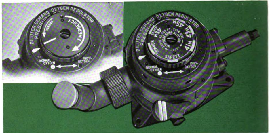
Fig. 2—The A-14 Diluter Demand Pressure Breathing Regulator with dial face used for pressure breathing. Insert shows reverse face of dial for use as a simple diluter demand regulator. Dial disk can be quickly reversed by removing two small screws.
