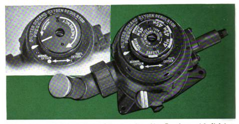
Fig. 2—The A-14 Diluter Demand Pressure Breathing Regulator with dial face used for pressure breathing. Insert shows reverse face of dial for use as a simple diluter demand regulator. Dial disk can be quickly reversed by removing two small screws.
