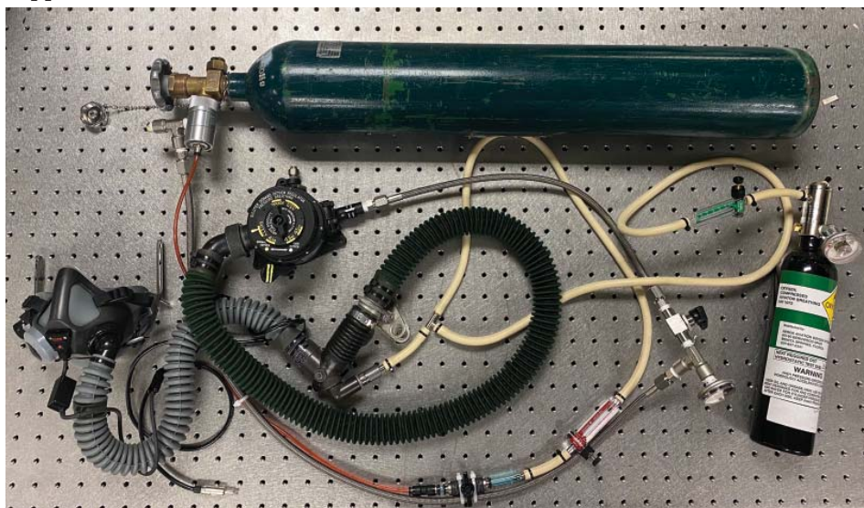
Above: Author after the flight. Photo by Britton Bluedorn. Left: Oxygen circuit showing 22cu-ft bottle, A-14 regulator, MBU-20/p mask, fixed flow system, and bailout bottle. Below: A-14 diluter-demand pressure breathing regulator (Fluid Power, Inc.).
