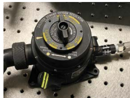
Above: Author after the flight. Photo by Britton Bluedorn. Left: Oxygen circuit showing 22cu-ft bottle, A-14 regulator, MBU-20/p mask, fixed flow system, and bailout bottle. Below: A-14 diluter-demand pressure breathing regulator (Fluid Power, Inc.).
