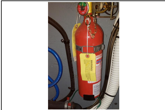
Fire Extinguisher Engine Halon 1301
