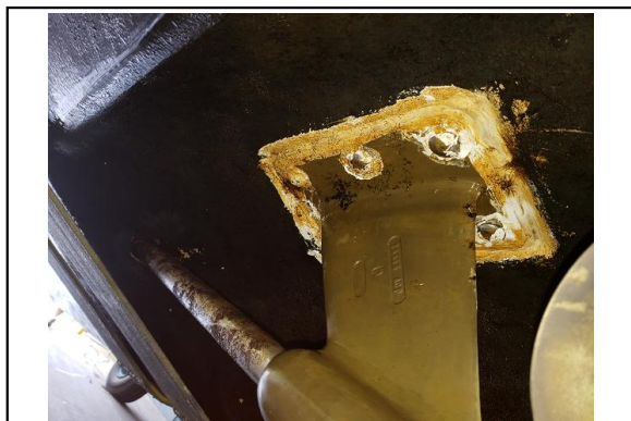
Bottom Prop Strut has had Maintenance
