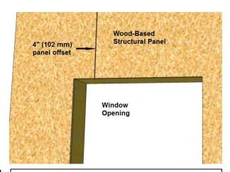
Detail 1, Reentrant Corner Detail
