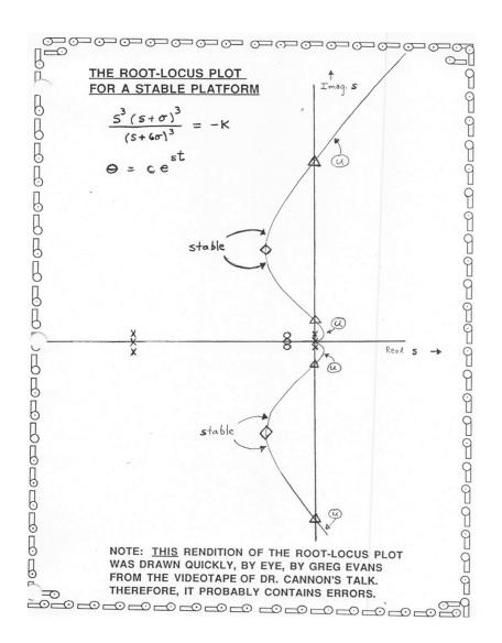
What you have is a characteristic equation at the top of the figure and what the characteristic equation has to do with is that the roots of that equation are the values "s" which will tell one how the system will behave.
