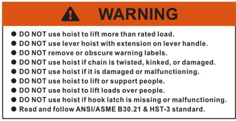
Figure 1 Warning Label on lever hoist's gear cover (shown larger for legibility)
