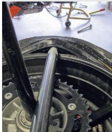
With the bar's 41" length, tremendous leverage can be exerted against a stiff/stubborn sidewall. Here's the demount tip in action, just beginning to pull off the first bead.
