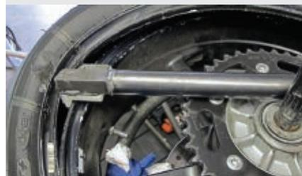
The bead is slick with tire paste, so the angled steel portion of the mounting tip smoothly guides the bead from above to below the rim edge.
