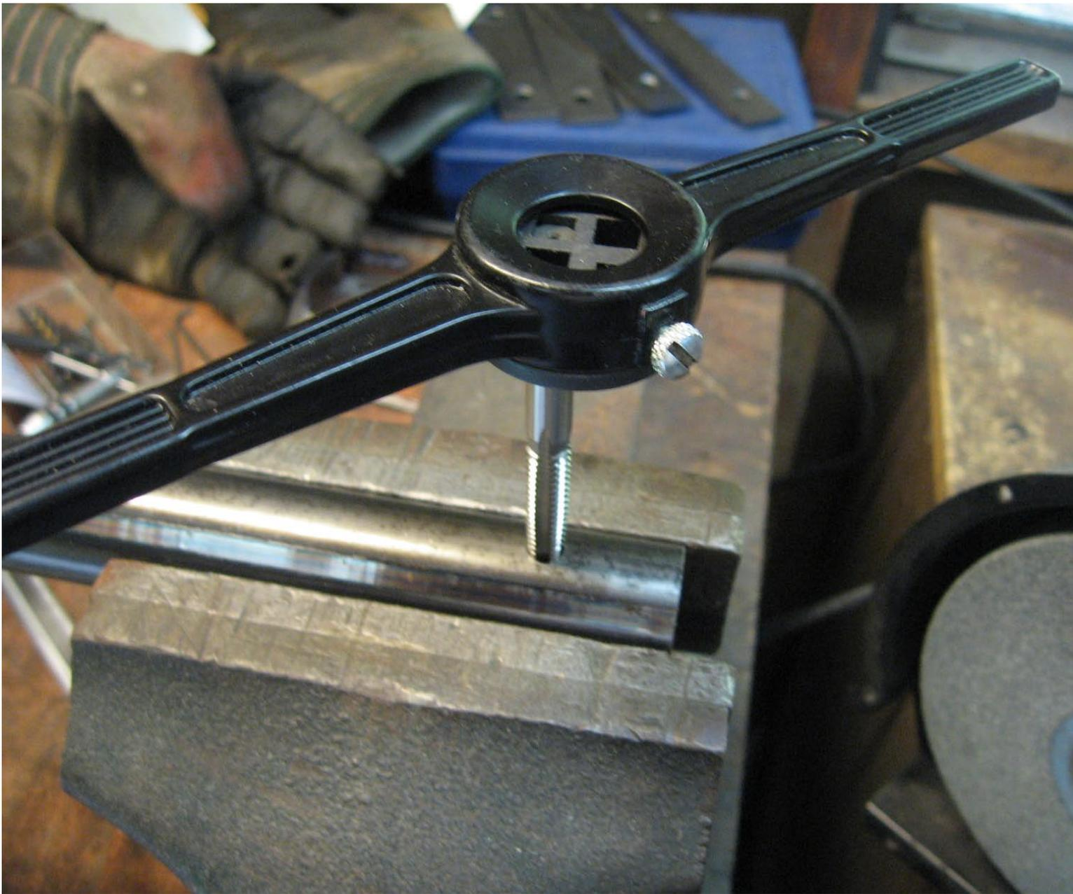
After removing the tap take your shiny new demount tip and insert it in the end of the bar, being careful to line up one of the holes on the tip with the hole in the tire tool. You know the hole you just drilled and tapped. Next tap your tip down into the bar until the shoulder of the demount tip is flush with the end of the tire tool. Note: to make tapping the demount tip into the end of the bar easier you can spray the demount tip with a shot of silicon or WD40. Just a little will do!
