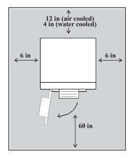
For machines without legs: For proper sanitary operation, its necessary to seal the machine to the counter to prevent liquid spillage on adjacent surfaces of the countertop from passing underneath the machine.
