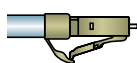
The LC connector is a small-form-factor fiber connector that features a ceramic ferrule. It looks like a mini SC connector.
