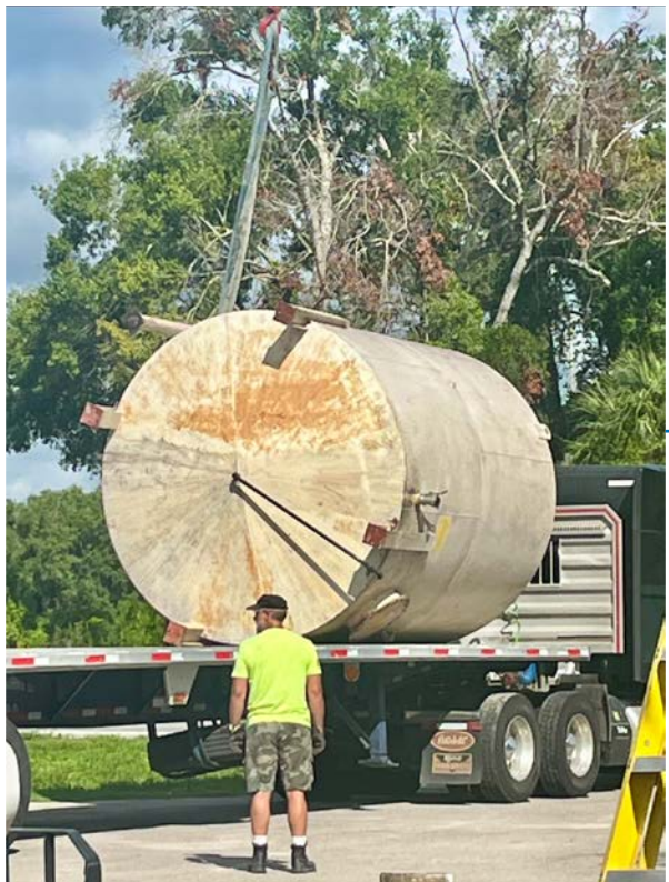
After the bulk oil tanks from Maassen Oil Company are moved to Florida’s east coast, they will be sandblasted, the welds checked and repaired if necessary, repainted, and shipped to north Florida. Photograph provided.
