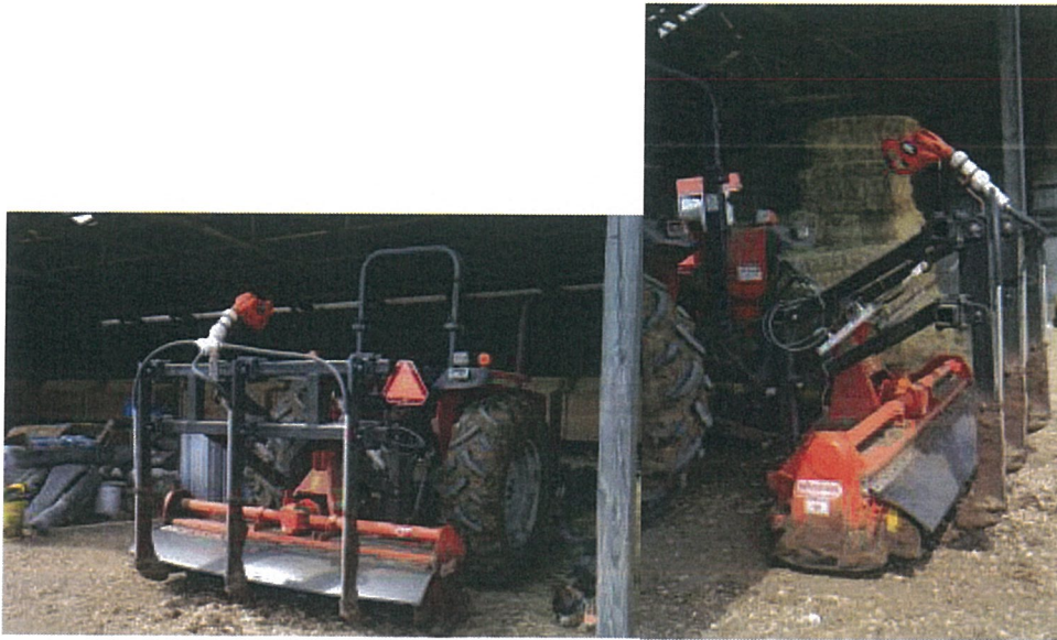
Plate 26-27: Cultivator used to add oxygen to the compost system
