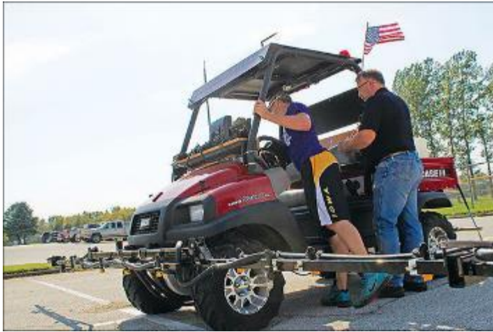
Figure 4.1.2 Prof. Kevin Butt with a student demonstrating a GPS enabled small Case ATV equipped with auto shut-off sprayer boom and auto-steer.
