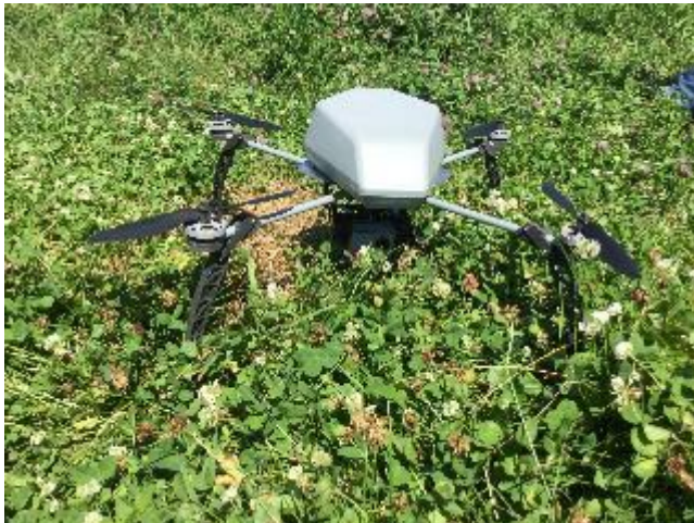
Figure 4.2.2 A quadcopter drone fitted with an IR camera. This type of drone does not have geo-referencing capability.
