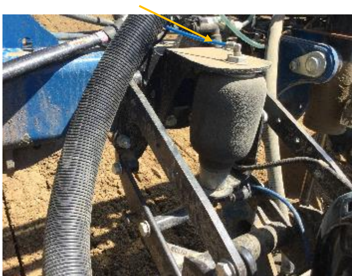
Figure 3.3.3 A pneumatic down force unit (shown by arrow) enabling an 'on the go' variation in the force applied to the coulter to control the depth of seed as it is planted.
