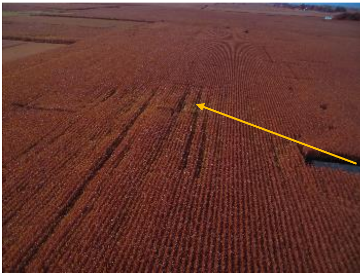
Figure 4.2.6 A near IR image of a field of maize taken from a quadcopter UAV. The arrow indicates areas of compaction that are difficult to spot using a camera using the visual spectrum.
