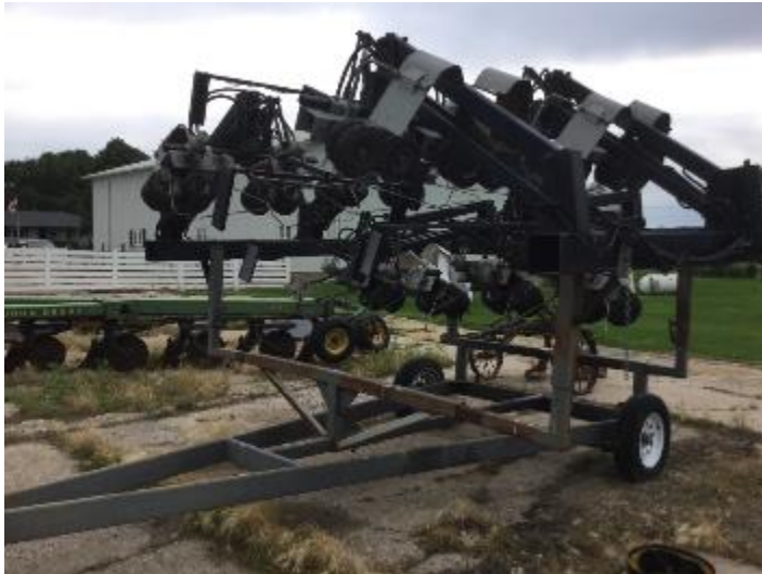
Figure 2.4.3 A detassler used to remove the male reproductive organs of the maize plant.
