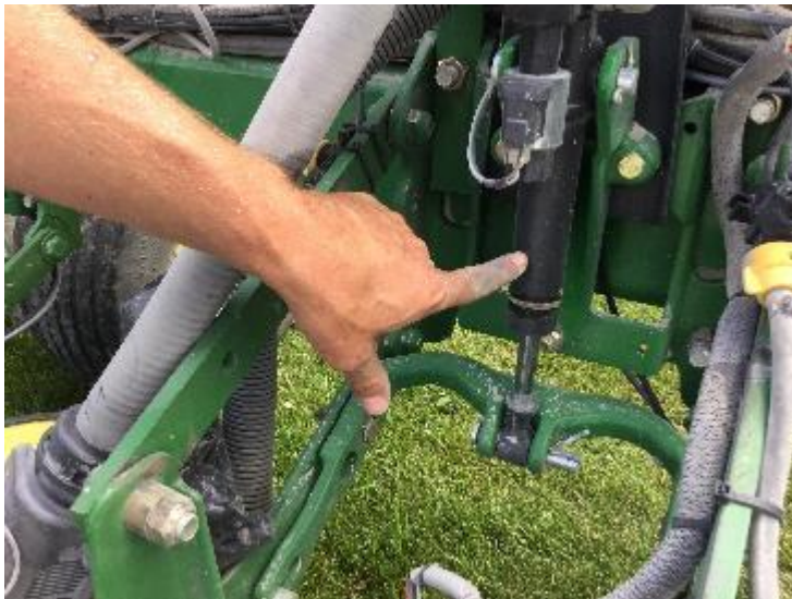
Figure 3.3.4 A hydraulic ram used to apply down force to a row in a John Deere planter.
