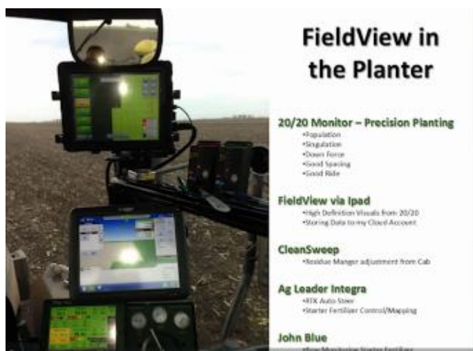
Figure 3.3.3 The use of Fieldview 'on the go' information system that is able to relay on tractor and implement performance during operations.
