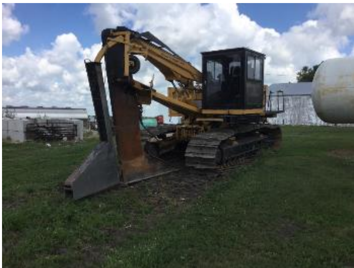
Figure 2.3.3 A trencher used for the installation of perforated pipes.
