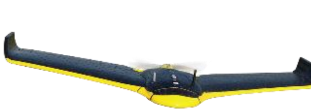
Figure 4.2.3 A fixed wing drone made by eBee fitted with a NVDI camera similar to the one used during the demonstration. This type of UAV does have geo-referencing capability. After: www.farmsolutions.com
