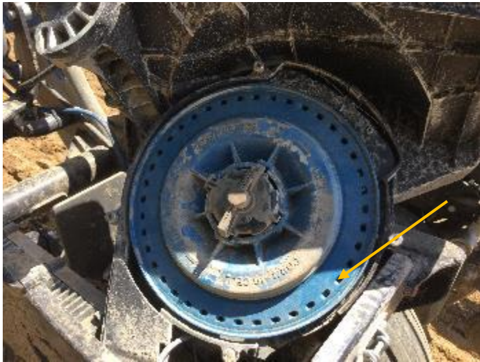
Figure 3.2.2 A vacuum disc used to ensure that a single seed is planted during any one given plating event. The arrow indicates where the seed is 'fixed' prior to being dropped onto the coulter during planting.
