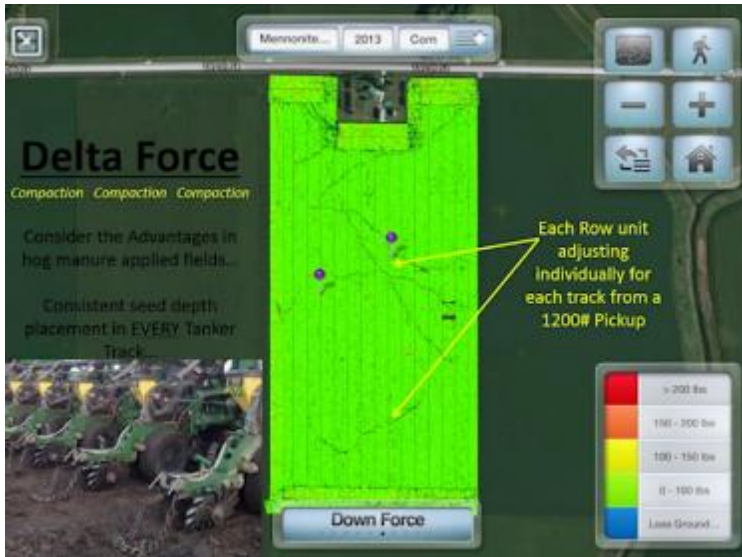
Figure 3.3.2 The down force for each row can be independently adjusted according to need using Delta Force. This is similar to products made by Kinze and John Deere.
