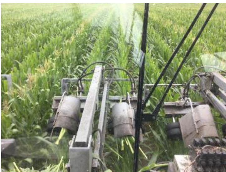
Figure 2.4.4 A detasseler in operation. The rubber 'wheels' placed either side of the maize plant rotate and sever the tassel from the main stem.
