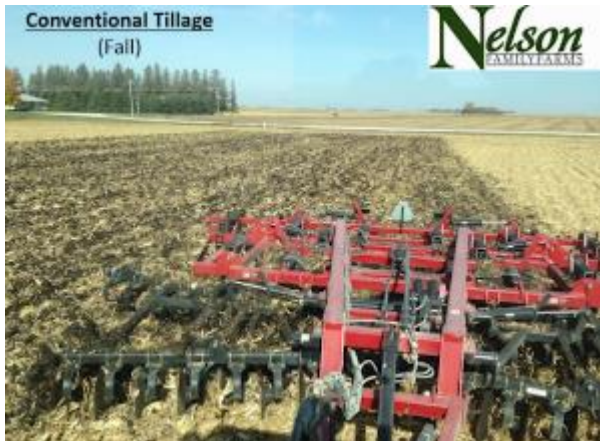
Figure 2.1.3 Conventional or reduced tillage system used in lowan cropping systems during the Autumn. This is a combination cultivator using discs and aggressive tines.
