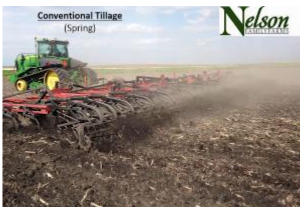
Figure 2.1.4 Conventional or reduced tillage system used in lowan cropping systems during the Spring. This is a combination cultivator using tines, spring tines and packers/rollers.
