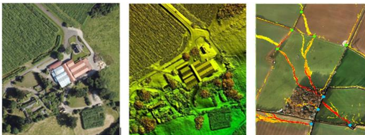
Figure 8: Comparison of an ordinary photograph compared to LiDAR (Van Rees, 2021) and example of identified hydrologically sensitive area map (Thomas et al., 2016)
