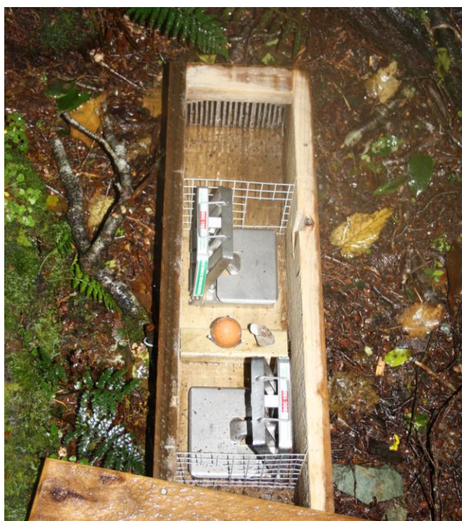
Figure 3 Double set DOC trap showing internal baffles and egg & rabbit meat bait
