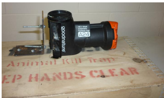
Figure 14 A24 retro-fitted to a DOC trap wooden box
