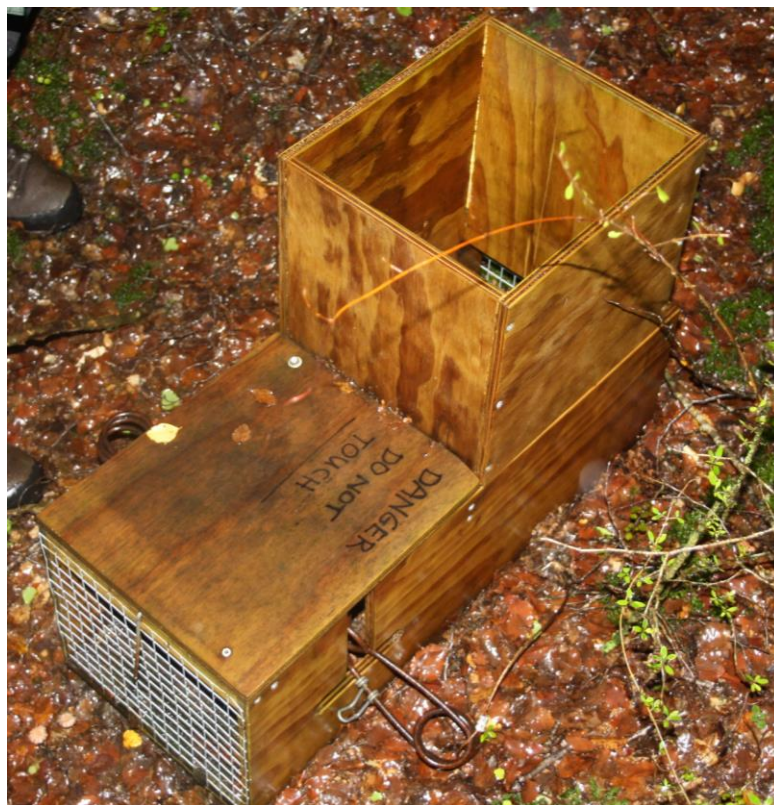
Figure 4 'Chimney' cat trap using Belisle Super X 220 traps
