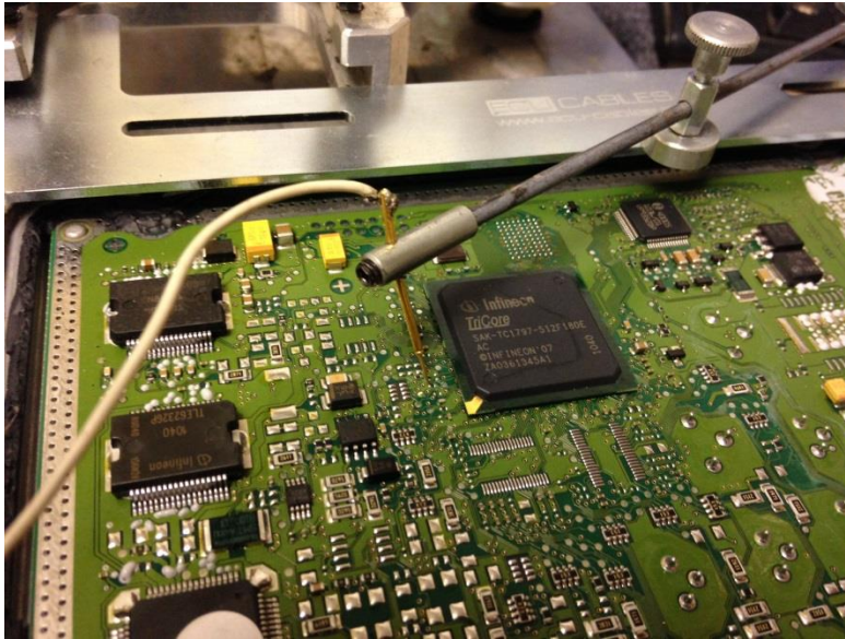
Probe showing bypassing tricore chip. (This process carries more risks than other methods due to the invasive nature of the process)
