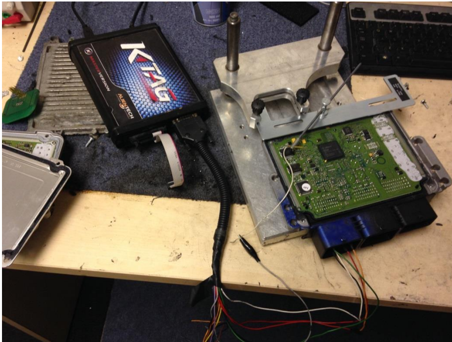
Above showing ECU open anti tamper tricore remapping. Note the grey wire bypassing anti tune microprocessor which is the large black microprocessor roughly middle upper part of board
