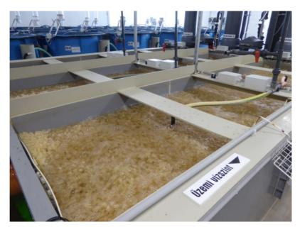
Fig. 3.5 Biofilter tank, HAKI
