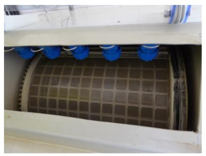
Fig. 3.4 Mesh filter drum
