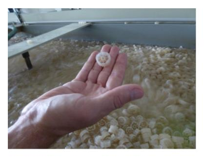
Fig. 3.6 Biofilter close up, HAKI
