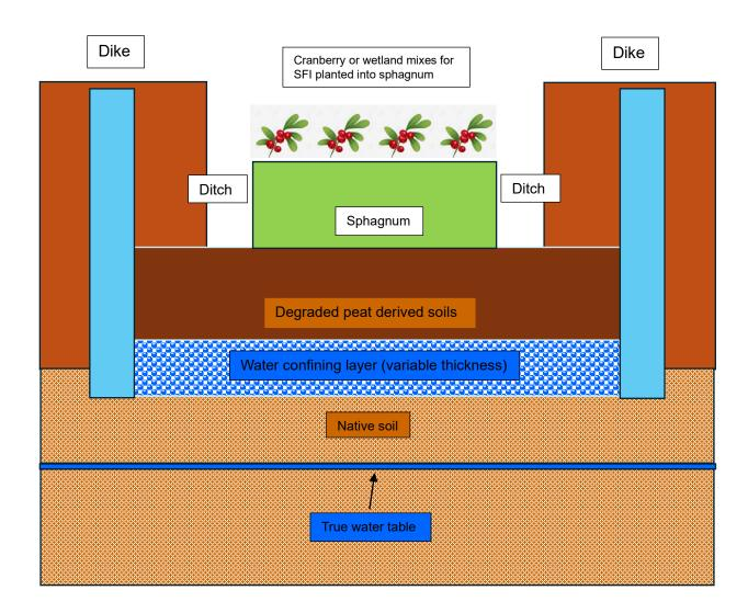
Figure \*\* Diagram showing the construction of a cranberry bed on peat in a system of intercropping with sphagnum (in green).
