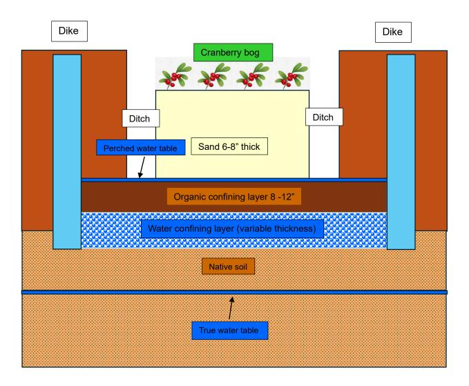
Figure \*\* Diagram showing the construction of a cranberry bed on peat with associated sanding layers similar to those seen at Lake Nokomis, Wisconsin.
