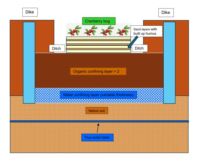
Figure \*\* Diagram showing the construction of a cranberry bed on peat with cranberry planted into sphagnum.
