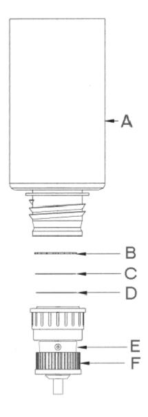
Figure 1 – Components of the Vacuum Filter Funnel and their proper orientation and assembly. A – Funnel, B – Filter Retainer Ring, C – 47mm Filter Membrane (not included), D – Membrane Support, E – Base Unit with Vacuum Port, F – GL-45 Cap Closure
