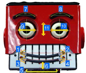
Fig. 2. DOF on Melvin’s face parts into smiles, frowns, etc. Using these DOF, in the appropriate directions, are thus a good choice for AU 12 (Lip
