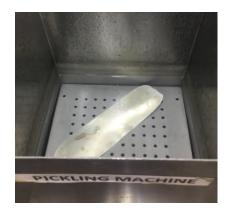
• Place it in a warmed pickle bath for 5 minutes, using a freshly mixed solution of pickle is best because it will more quickly remove the copper oxides.
