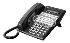
The **34-Button Display Telephone** features 24 Programmable Function Keys.
