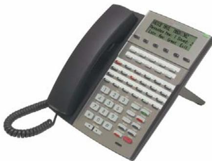
The 34-Button Display Telephone features a large 3 line-by-24 character backlit alphanumeric display with 4 Interactive Soft Keys for intuitive feature access. It also provides 10 Personal Speed Dial bin keys, 24 programmable Feature Keys and 12 fixed function keys for streamlined operation. Additionally, this telephone offers a backlit keypad, a headset jack, and built-in speakerphone. Unique features include dual LEDs, built-in wall mounting, and an innovative two position angle adjustment.
