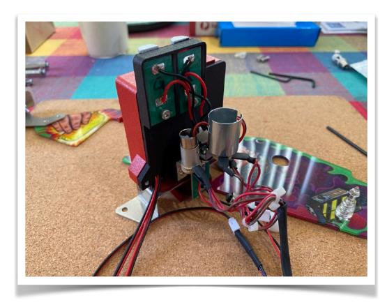
Then install the PCB lead from the back cover into the second adaptor lead of the Flasher Socket. Next feed the back cover around the sockets and back of the mod and line up with the hole on either side of the Stainless Steel bracket using the original black screws to secure.
