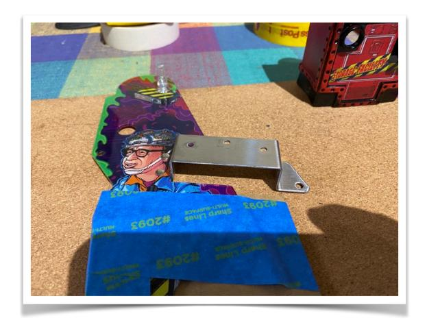
Now you will have a game cable with 3 sockets attached to posts, so now remove the sockets from the posts and bag the posts and screws. Note: put some tape on sockets or write on the socket a **R** (**Red**) and **G** (**Green**) so when reassembling you get the sockets on the right side (but if you get it wrong it will be easy to swap cables).
