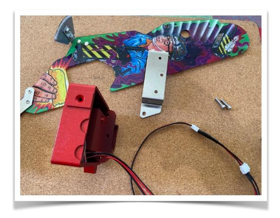
Then slide the cabinet over the stainless steel bracket and locate over the holes and insert both bolts but get both bolts started and then secure. Securing and locking one bolt down may make securing the 2nd bolt difficult.
