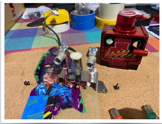
Now remove the  $2 \times posts$  as well as the large flasher socket. Though when turning the plastic over take care to not break the plastic. I secured the plastic to a piece of cardboard with some painters tape to strengthen and support the plastic.
