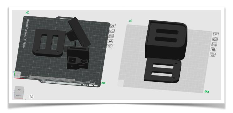
On both plates is a thin base plate in which you only need one but one is for low profile bolts and the other is for countersunk bolts - simply delete the one you do not need.
