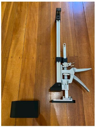
the front of the cabinet and the larger booster base is for use at the back of the cabinet. Simply drop the jack and it's thin base into the booster base and slide into position.
