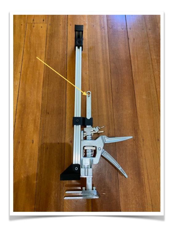
5. You can either double side tape the thin base to the bottom of the jack, or bolt on with any bolts you have on hand - approx 20 mm long.
