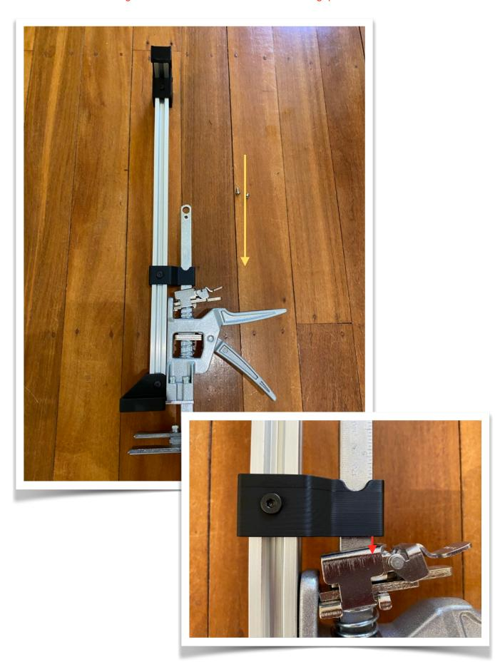
4. Lastly re-install the limit screw at the top of the vertical jacking arm as this limits how high the Centre Jack Lift Arm Slide Guide can go.
