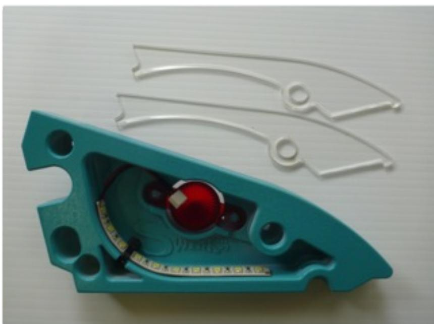
Note: since some people have expressed a desire to experiment with different colour LED's (refer page 17 for purchase links to pick a new / different colour), the pre-installed White LED Strip will be held in place but can be easily swapped over in less than 5 minutes at a cost for \$5 USD for a different colour strip from Comet Pinball.
