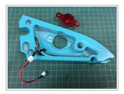
Then locate the Clamp Plate into the mod - note: before installing you first need to tap the hole in the centre hole refer to Section 3.
