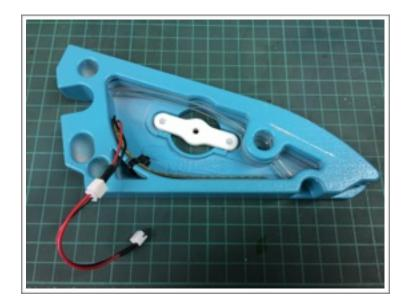
Then for the v2.0 owners place a small dab of hot glue over each locator pin to lock in place. This is done mainly so when you loosely install the signage you can swing it out of the way making the installation of the mod back into the game easier and then swing the sign into the preferred position and nip up the centre screw knowing that the Clamp Plate will not drop out mid way through the install. The photo shows V2.0 owners what the small dabs of hot glue will look like.
