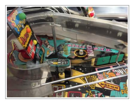
• Remove the centre sign post bracket (the one with the 'super jackpot', 'jackpot', 'rescue' and 'multi-ball restart' plastic attached to it). Keep the nut as you'll be re-attaching it after you complete installing the new Snackbar Base Plate.
