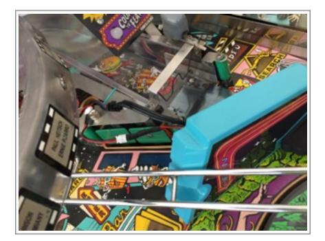
• Now with the Snackbar Top secured to the magnets lift the play field again and plug the mini controller into the power lead plug and secure the mini controller to the main harness as shown so it can not vibrate.
