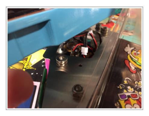
• Then the Snackbar Top simply drops in place on to the magnets locking the mod into place.
