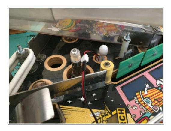
• Install the SS base plate into the location over the 3 current screws. Refer to the photo below.
