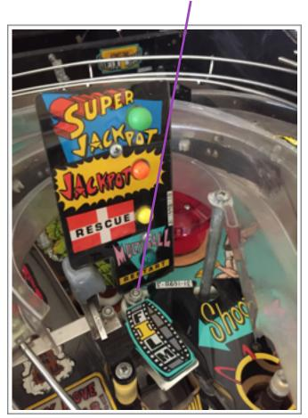
• Remove the 2 x 5/16" nuts and the phillips screw securing the original Snackbar plastic in place, resulting in what is shown below.
