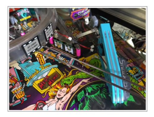
• Then when you have fed the wiring into the cavity try and feed excess into the large spare playfield hole and where possible keep away from globes.
