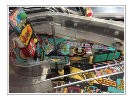
• Remove the centre sign post bracket (the one with the 'super jackpot', 'jackpot', 'rescue' and 'multi-ball restart' plastic attached to it). Keep the nut as you'll be re-attaching it after you complete installing the new Snackbar Base Plate.
