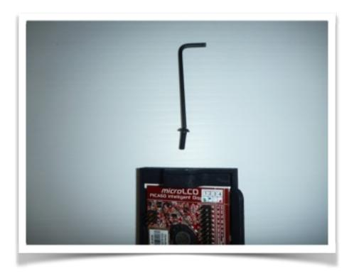
• The 2015 screen will need 2 basic jumper wires from any electronic shop for a under \$0.50 and wired in to the ground and 5 vdc pins as per below.
