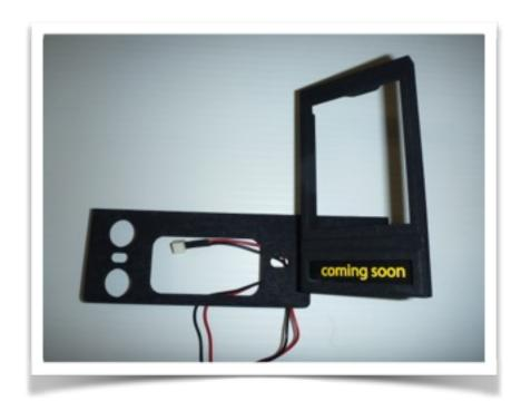
• I would recommend programming the screen prior to installing so refer to pages 4-6. Then install the screen, simply drops into 2 dedicated slots on the bottom behind the "coming soon" message.
