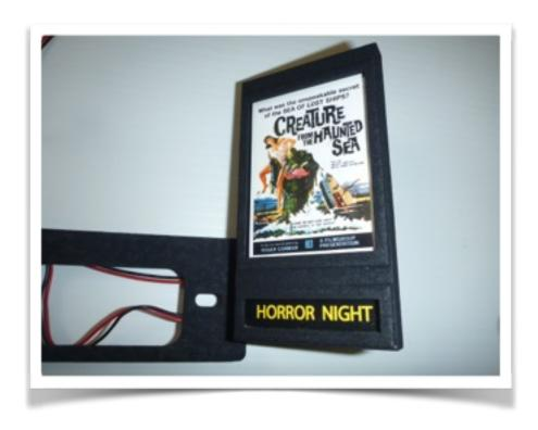
• Install the Poster retainer into the back of the frame. The retainer holds the poster in place but also houses the led strip in place minimising the light blasting out the back. The hole in the back is for an optional wire access if you decide to use a pad SMD led.
