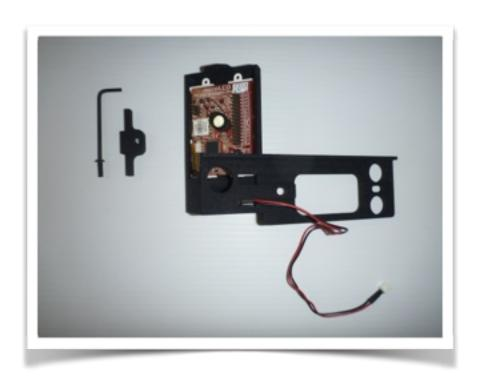
• Then install the LCD retainer bracket at the top and this as well as the main frame body is universal for the 2015 and the soon to be released Gen4 2016 2.8" screen (only difference is the back is more compact).
