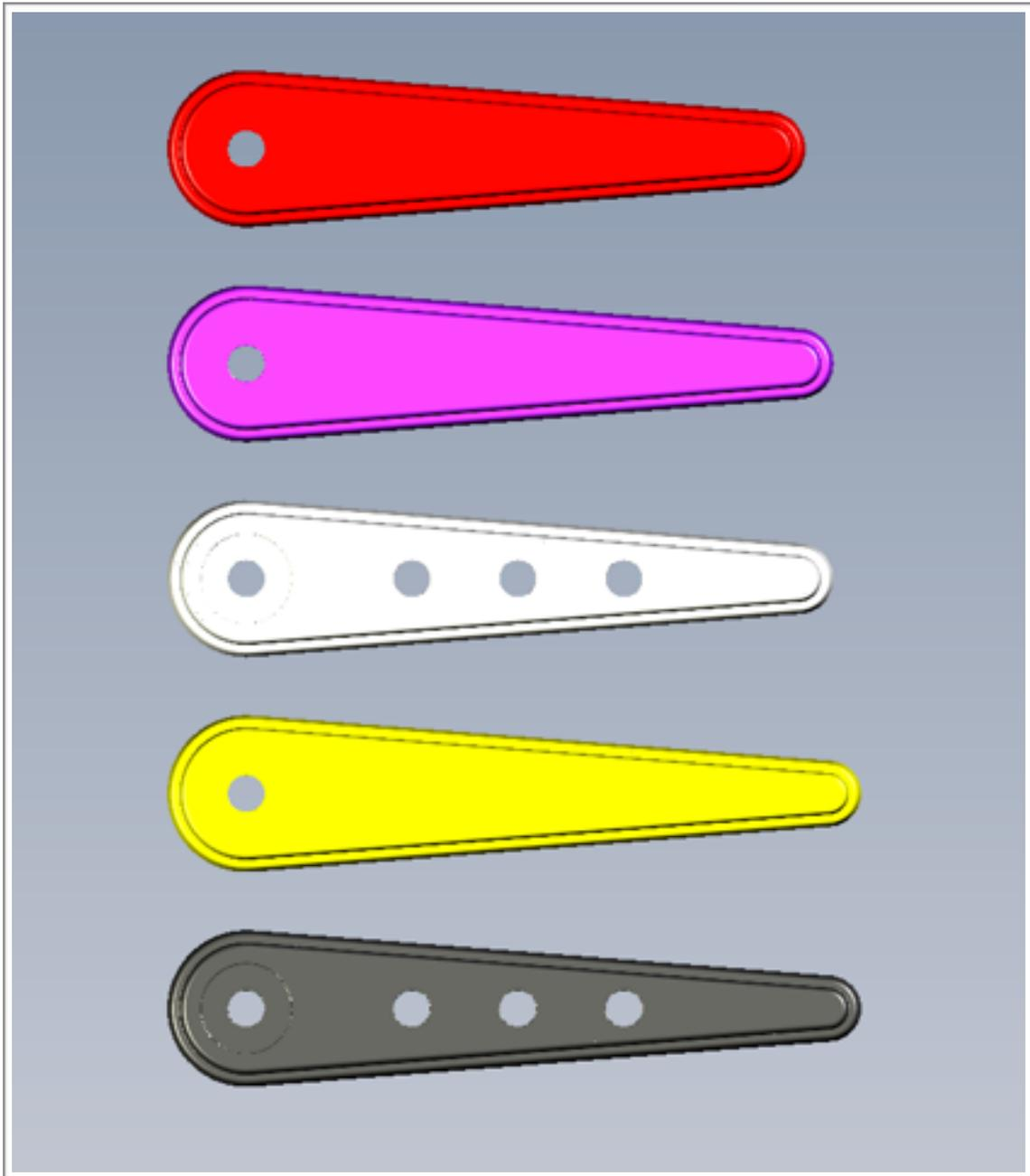
**CSF#4 - Bat** and **CSF#6 - Bat** require the **CSF#11 Fake Bulb** to be inserted for that PKE Meter look. The fake Bulb set but be held in place either via glue or taping the 2 holes in the bats. So to prep the bats for Fake Bulb sets screw fastened you tap M3.
