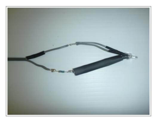
• Now heat shrink and divide the cable as shown ready for installation into the whomobile.
