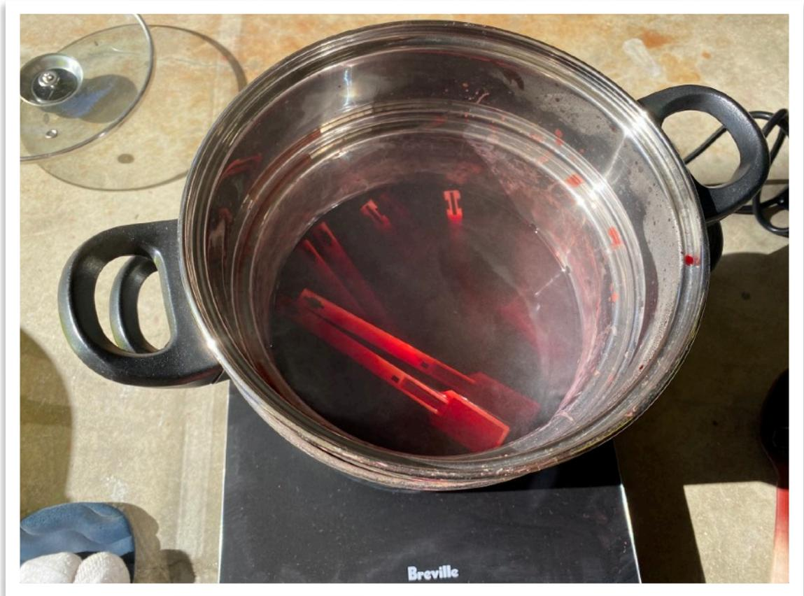
Once happy with the colour, turn off the portable cooker and lift the chip basket out of the pot and scoop the plastic parts carefully as they will be very hot and put into you still hot water in the spare bucket and let them sit there for another 15 minutes.
