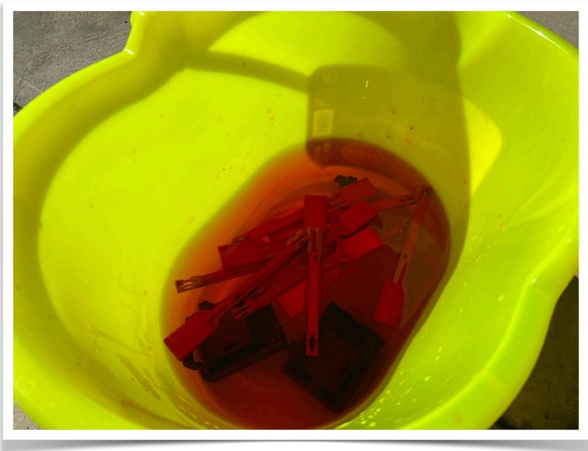
Then after 15 minutes remove one at a time and wash clean with a hose or at a sink and then I also use compressed air to blow off the water off the target face as they can get droplet stains if just left on a drying rack / saw horse after hose rinsing.
